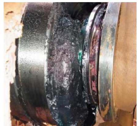
After 40 months operation the housing cavity grease was substantially free from iron ore contamination
