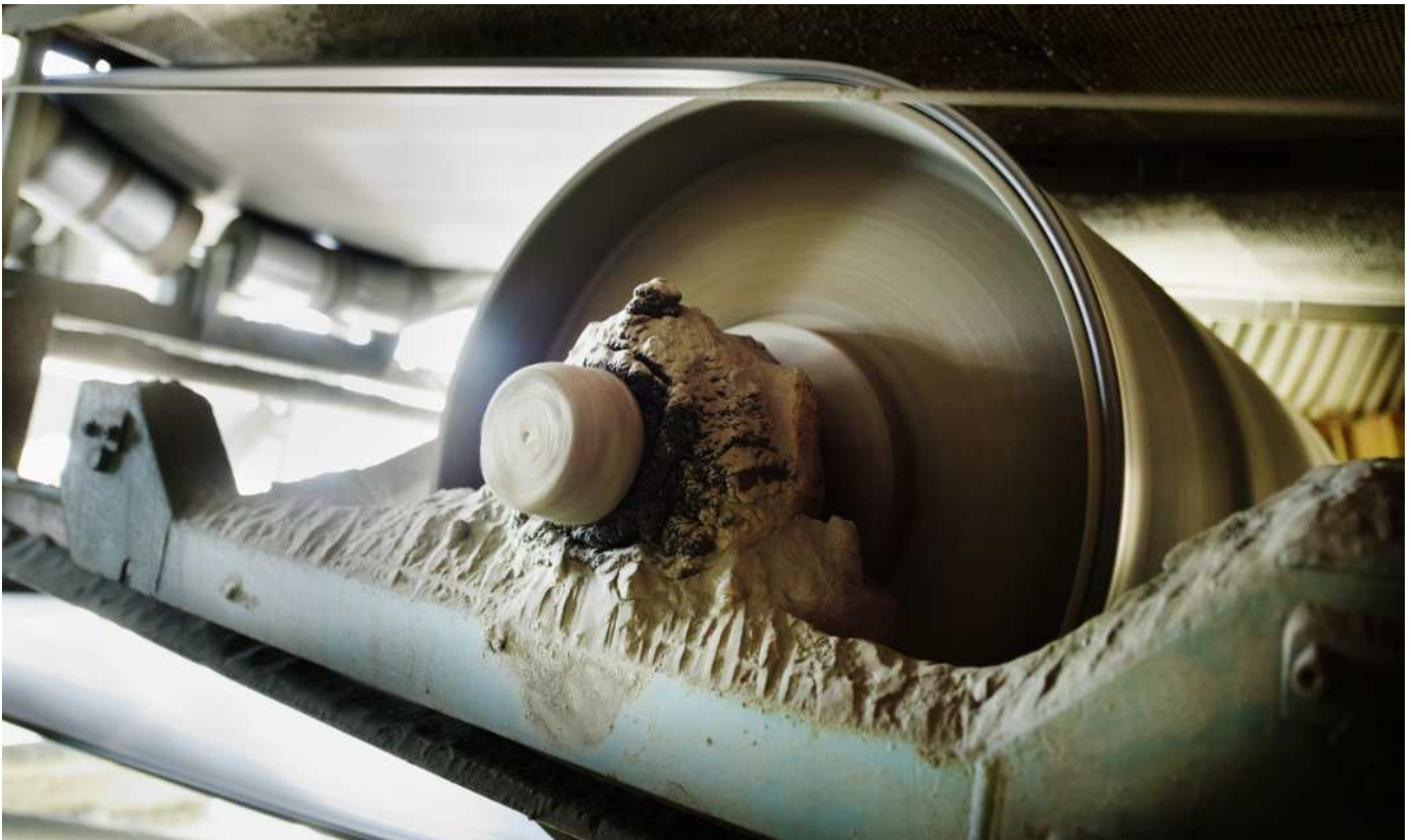
51% of bearing failures are due to contamination and ineffective lubrication
