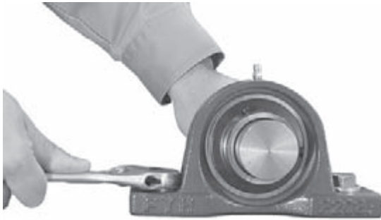
Fig. 14.4 Installation of setscrew units
