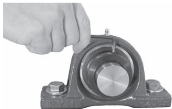
Fig. 14.10 Installing eccentric locking collar
